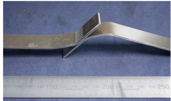
Figure 11 Successful hammer-S bend test result
