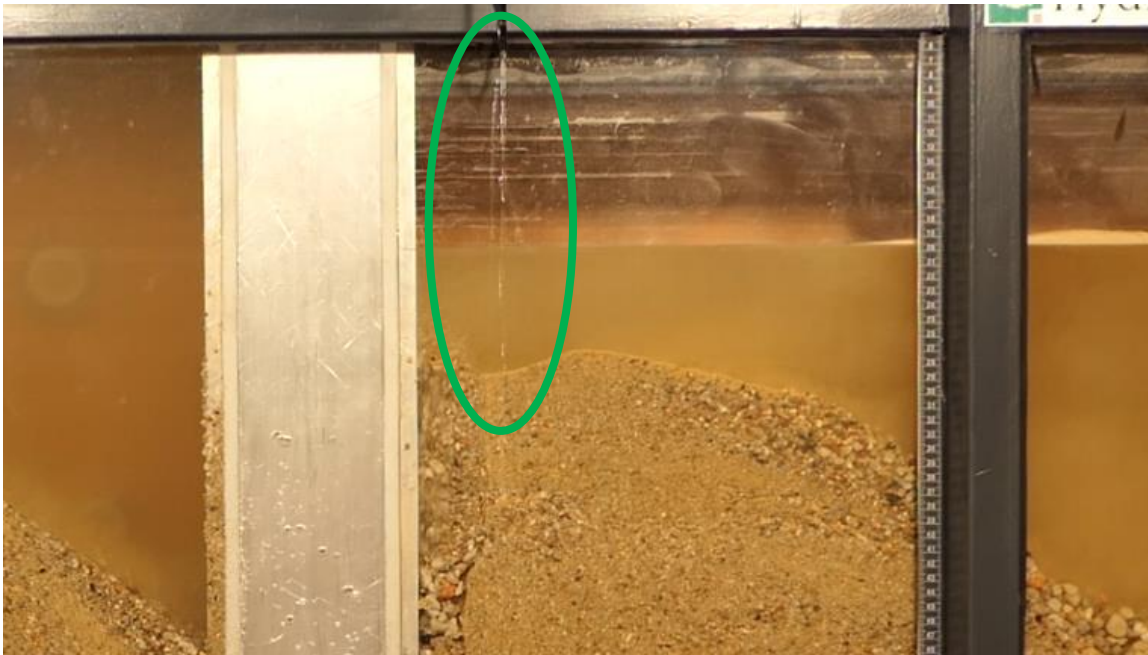
Figure 7.5: The existing leakage in the experiment
