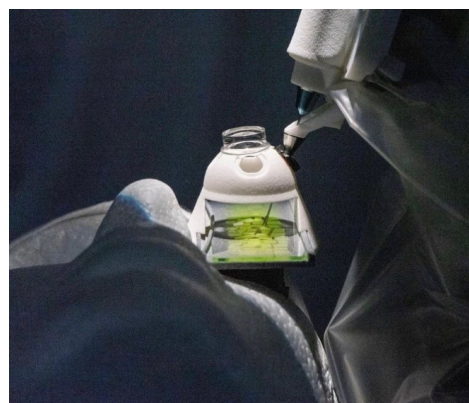
Figure 1. Practical training simulating epiretinal membrane peeling in order to familiarize the surgeon with the functionality of the Preceyes Surgical System (PSS). The phantom eye contained a gelatin layer with superficial embedded thin paper to be peeled during the training.
