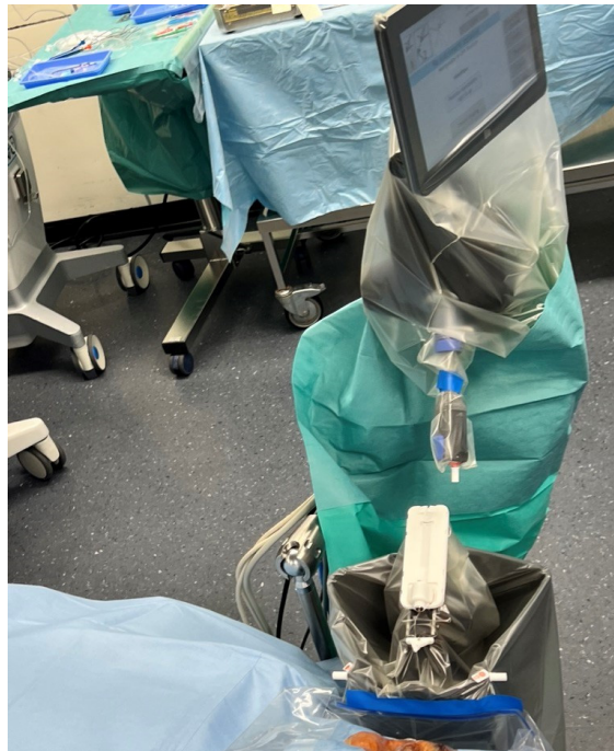
Figure 3. The draping of the PSS contains the instrument manipulator, trocar holder, motion controller, and cables. The extra draping, which maintains the sterility of the instrument manipulator during the introduction of anesthesia, has already been removed.
