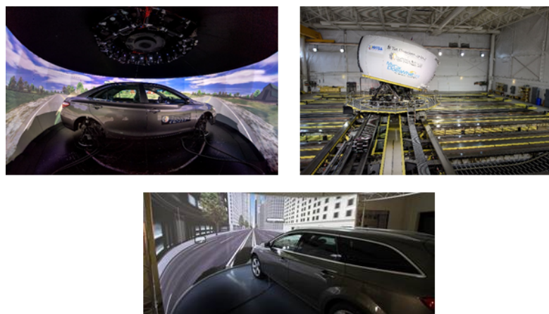
Figure 2. Photographs taken from the inside (top left) and outside (top right) the National Advanced Driving Simulator (NADS-1), a highly advanced moving base driving simulator at the University of Iowa, USA. The bottom image displays a more advanced fixed-base simulator that features the cabin of an actual vehicle, as setup at the Institute for Mobility (IMOB) at Hasselt University, Belgium.
