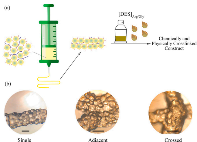
Fig. 1. (a) Scheme of 3D printing process based on jammed microgels, its extrusion and chemical crosslinking. Particle jamming occurs when the water content in the system decreases below a critical point in which the PGMA segments over the particles provide contact forces between the neighboring microgels. After extrusion, gelatin molecules (blue lines) convert to gel state and the strength of the material is increased. In the next step, [DES] Arg/Gly can be applied either in pure state or spraying aqueous solution to trigger chemical crosslinking reaction. (b) The images of the extruded ink under an optical microscope in three common positions used in additive manufacturing process. Scale bar is 200 μm.
