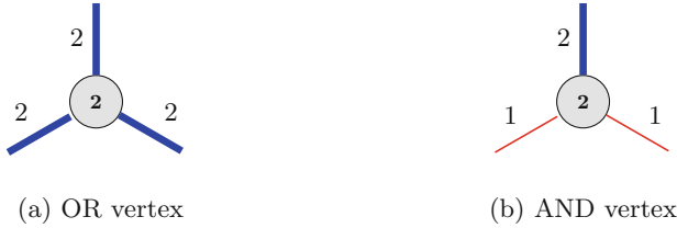
Fig. 6. The two vertex types from which a restricted constraint graph is constructed: (a) OR vertex and (b) AND vertex. Following the convention set in [13], as a mnemonic weight 2 edges are drawn blue (dark grey) and thick, while weight 1 edges are drawn red (light grey) and thinner. From [23]. (Color figure online)
