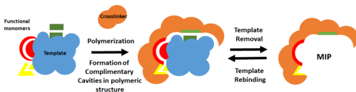
Figure 1: A generic schematic demonstrating the fundamental principles behind the synthesis and extraction of a MIP.
