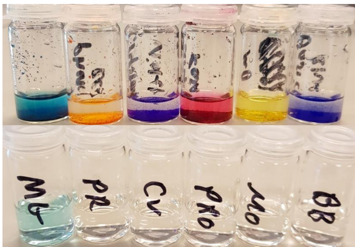
Figure. S4. SDC concept. MIP particles loaded with malachite green, phenol red, crystal violet, pararosaniline, methyl orange and basic blue (left to right) were incubated with 5 ml 2-MXP (1 mM) for 5 minutes (top). The particles were then filtered off and the resulting filtrates colour observed (bottom).
