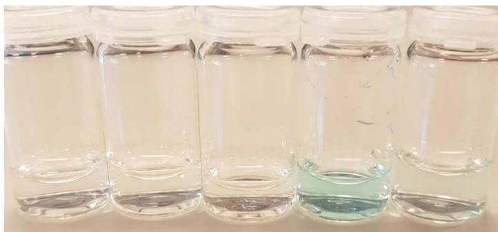
Figure. S5. SDC-concept. MIP-21, MIP-22, MIP-23, MIP-24 and MIP-25 (left to right) were preloaded with malachite green and incubated with 5 ml 2-MXP (1 mM), filtered and the colour of the filtrate observed.
