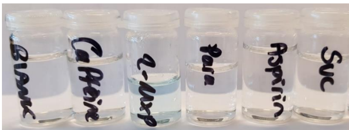
Fig. S8. SDC concept. Malachite-green loaded 2-MXP MIPs were exposed to a range of targets. The filtrate will only color when the MIP is incubated with its target as the dye is displaced from the MIP particles.
