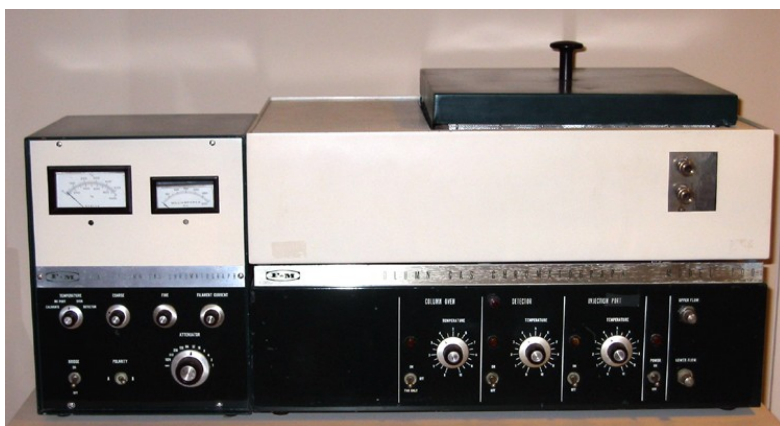
Figure 1 - Fe&M Model 700 Dual-Column Gas Chromatograph, ca. 1961 (Source: Courtesy of the Chemical Heritage Foundation)
