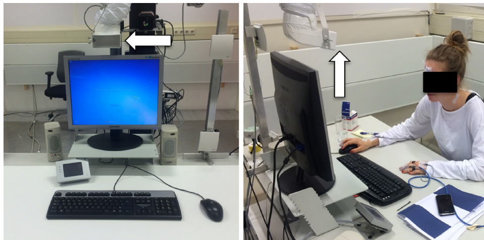
Fig. 2. Experimental setup. The white arrows indicate the outlet of the fan. The outlet position was adjustable in height and angle to individually direct the airflow onto the participant's face.
