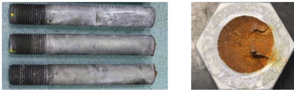
Figure 4. M52 class 10.9 bolt that failed in service due to delayed fracture.
