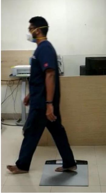
Figure 3. Plantar pressure measurements in walking (dynamic analysis)
