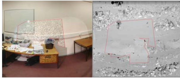
Figure 7.5: Structured light pattern projection results showing fewer errors in the depth map where the structured light is projected (inside the red line)
