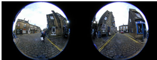
Figure 2.6: Two 180° hemispheres that can be used to create an omni directional image
