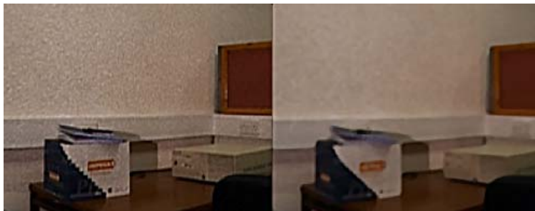
Figure 7.2: Showing the structured light pattern in an image (left) and after it has been removed (right)
