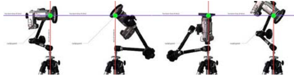
Figure 4.4: The multi-shot system, showing 4 of the 26 positions used
