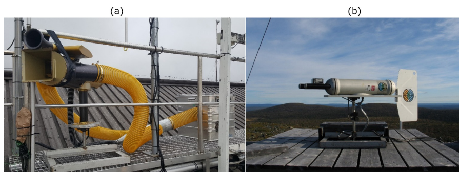
Figure 3. CAPS (a) and FSSP-100 (b) ground setups as installed on the roof of Sammallunturi station.
