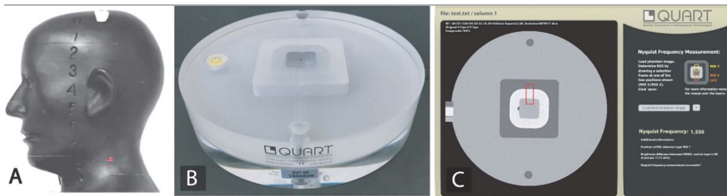
Figure 2. (A) Anthropomorphic RANDO RAN 102 phantom used for ED assessments. (B) QUART DVT phantom. (C) Analysis software window for calculating CNR.
