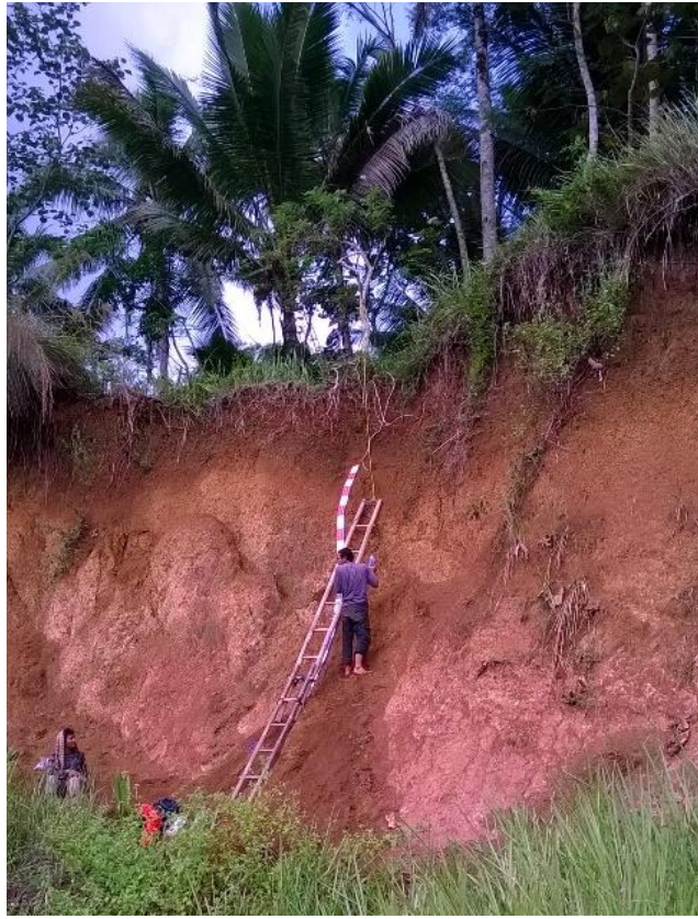
Figure 4.6 The thick soil layers in the Bompon watershed. The picture was taken on the Kalisari landslide site.
