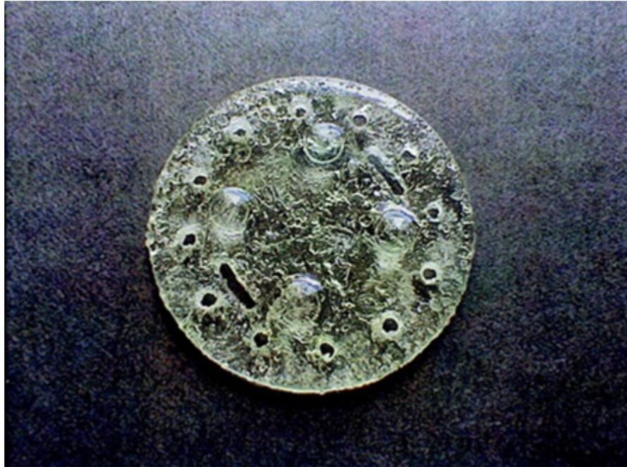
Figure 18. fabricated scaffold using SLA. Adopted from M. N. Cooke (124).
