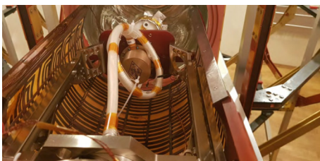
Figure 4. The Mars orbiter magnetometer sensor fixed at a mounting plate and ready to be pushed into the thermal box.
