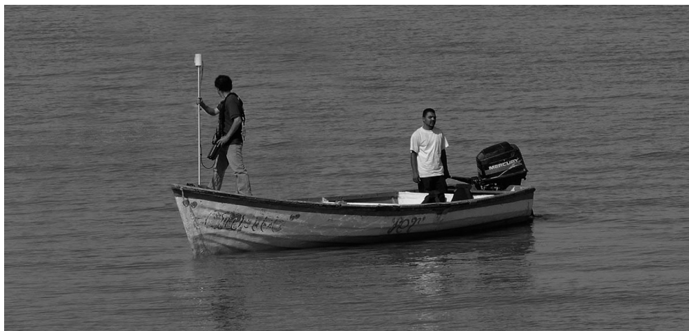
Figure 3. Surveying with the G856 precession proton magnetometer placed in the bow of a fiberglass boat.
