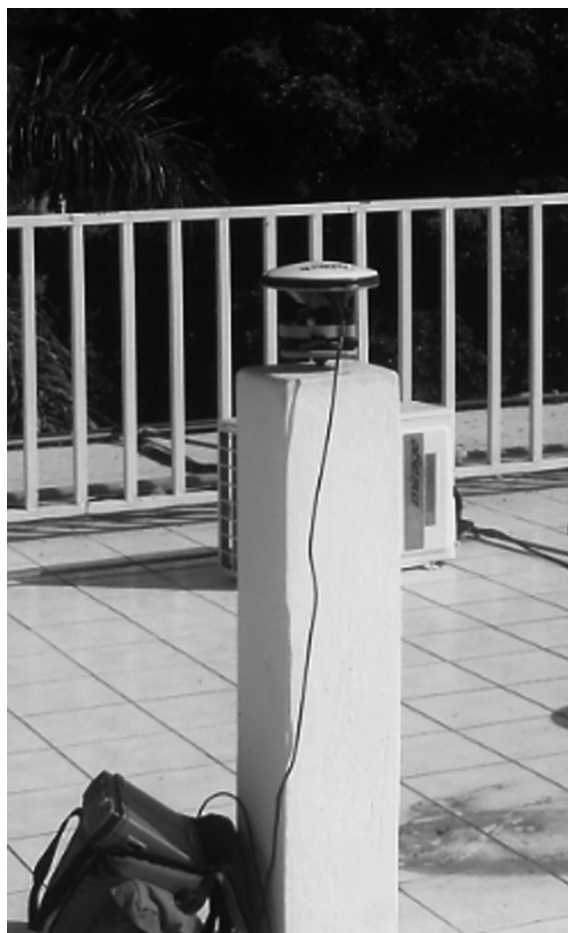
Figure 2. Monumentation of BASE 1 site, located on top of the FACITE building; UAS campus. GPS Receiver Ashtech Z-Xtreme with Ashtech (ASH701975.01A) antenna, collecting data on October 9, 2010.
