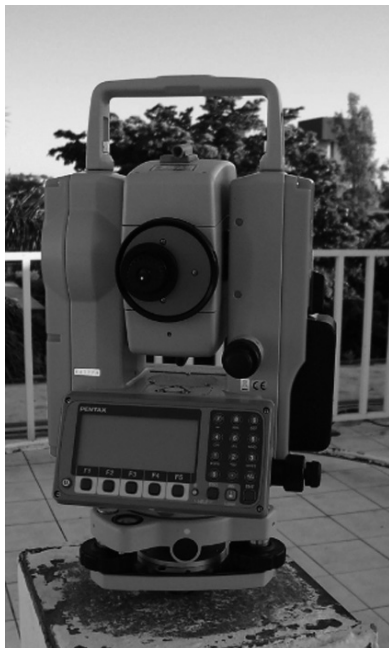
Figure 6. EDM measurements with PENTAX R-326EX at BASE1 site (see BASE2 in the background), performed on October 8, 9 and 10, 2010.
