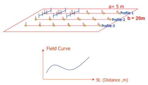
Figure 5. Profiling by schlumberger array
