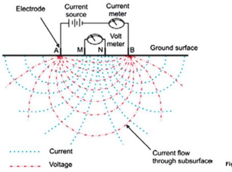
Figure 4. The basic principles of Schlumberger device
