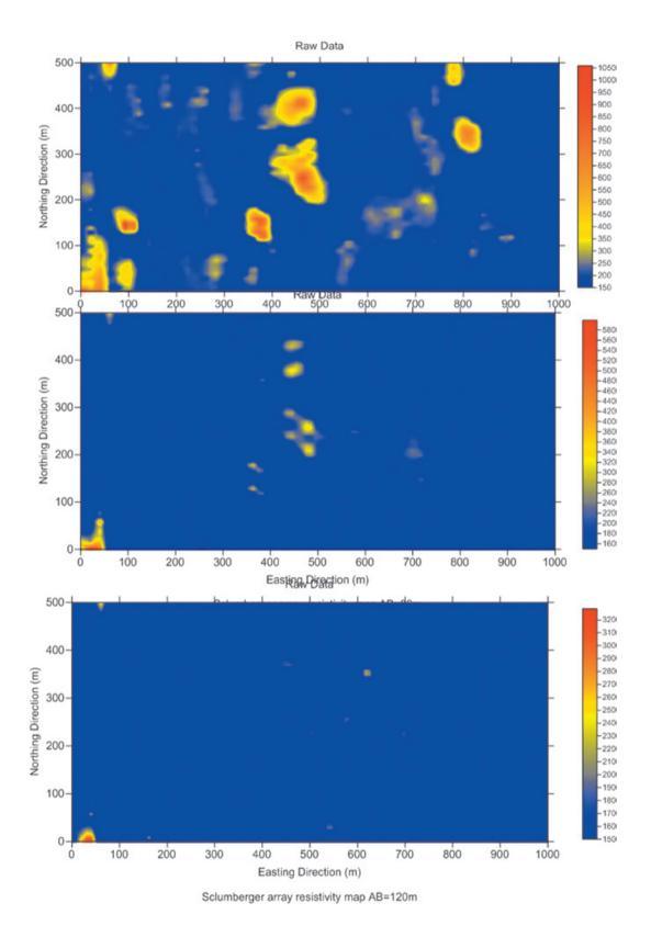
Figure 6. Maps of the apparent resistivity for various Schlumberger electrodes spacing (a) AB = 40 m (b) AB = 80 m and (c) AB = 120 m.
