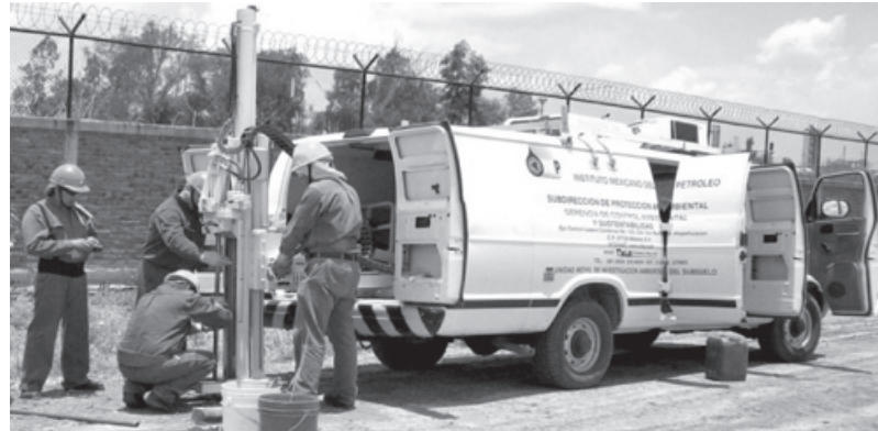
Figure 5. Geoprobe System used to collect soil and ground-water samples
