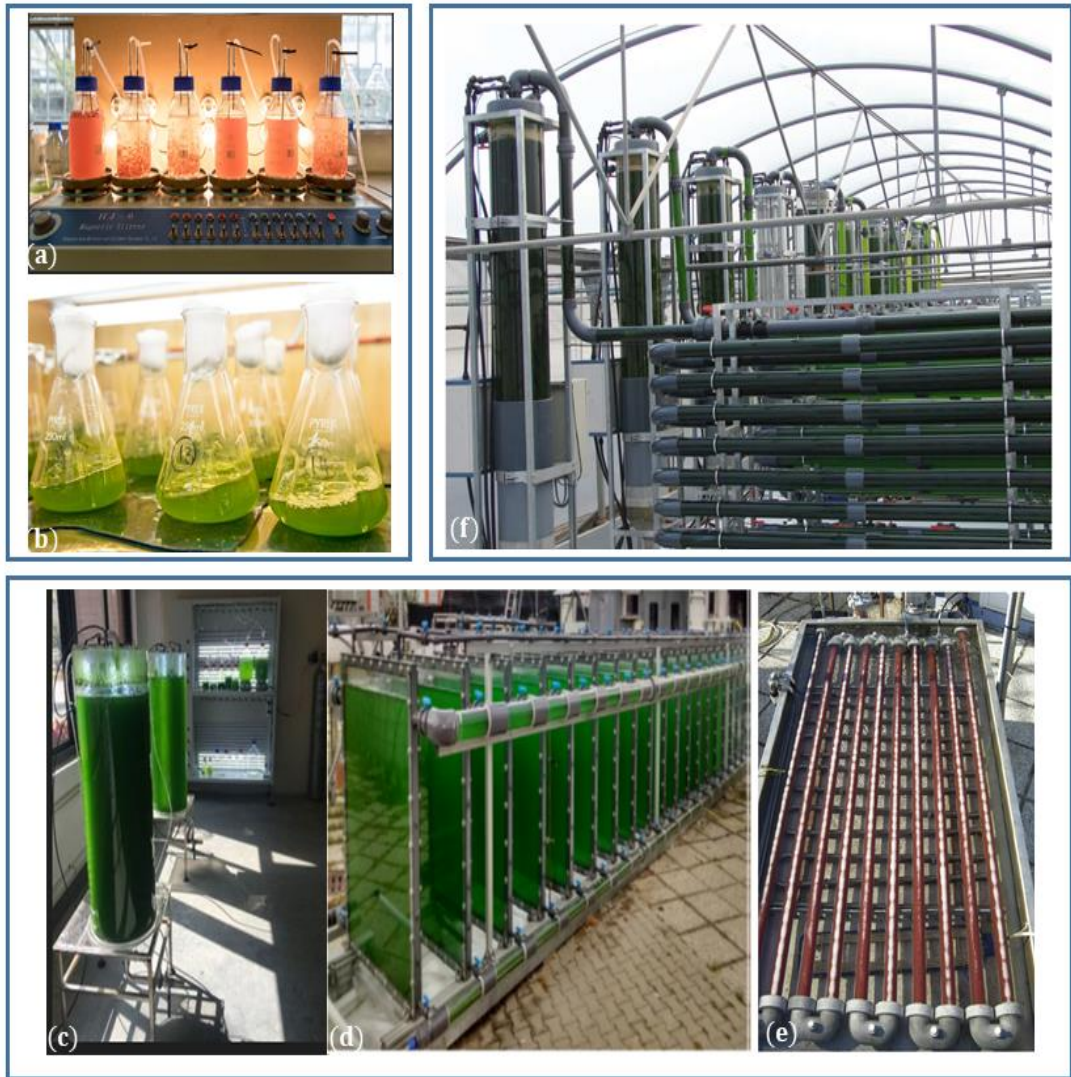
Figure 2.4: Various scales of closed PBRs: lab scale PBRs (a) to (b), pilot plant scale PBRs (c), (d) reproduced from Lindblad et al., [23] and (e) reproduced from Adessi et al., [19], and industrial scale PBR (f) reproduced from Yen et al., [46].
