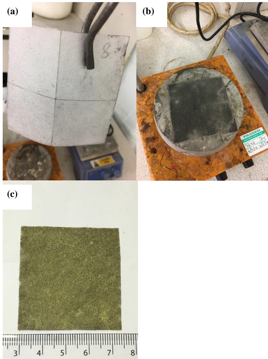
Figure 3-6. The nanoscale silver ink impregnated nonwoven fabric, (a) before thermal sintering; (b): during thermal sintering; (c): thermal sintered and cut into a smaller size designed for sensor fabrication.
