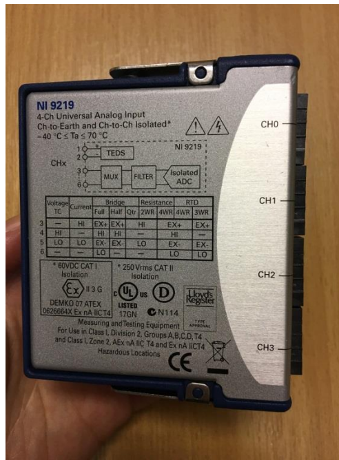
Figure 3-12. NI-9219 data acquisition card.
