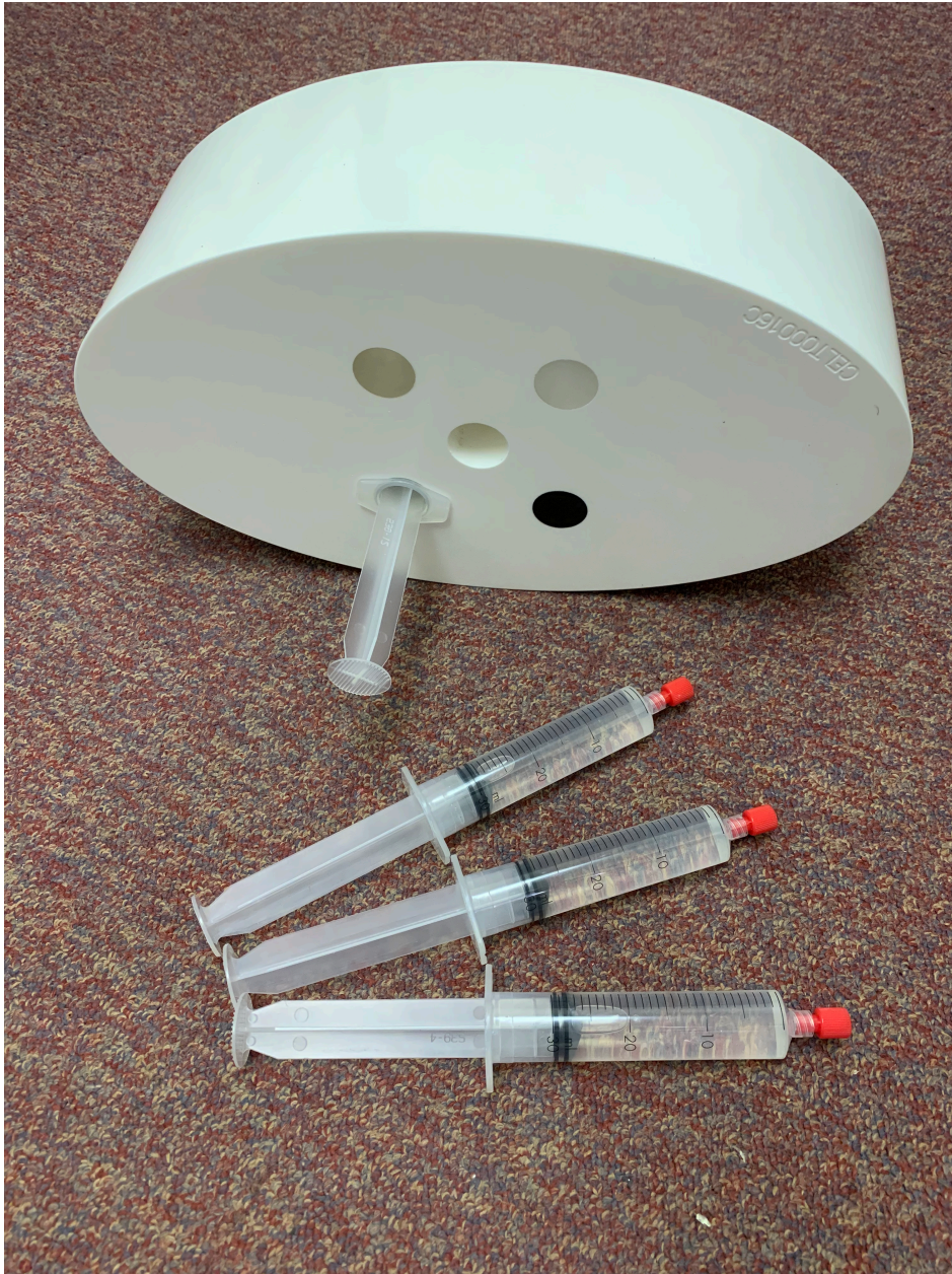
Figure 1 A photo with the section of the CeT phantom used, with locally produced iodine inserts
