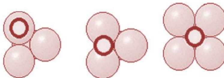
Figure 2.12: The three possible adsorption sites offered by the fcc(100) metal surface.
