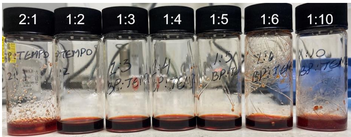
Figure 6.9. Image of BP:TEMPO mixtures with molar ratios from left to right of: 2:1, 1:2, 1:3, 1:4, 1:5, 1:6, and 1:10
