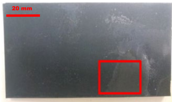
Figure 5.4 An example of coating damage during the icing test
