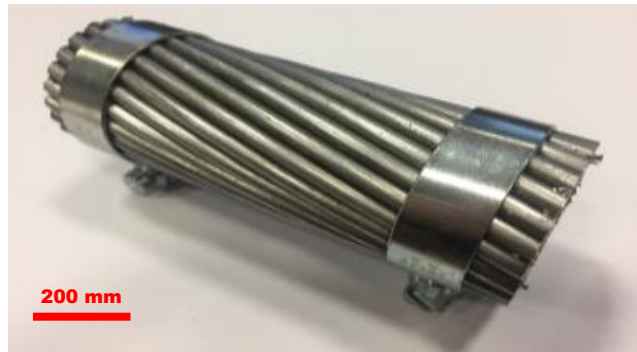
Figure 3.3 Image of an AAAC conductor line
