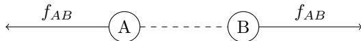
Figure 2.1: Two atoms A and B interacting with force f_{AB} which the machine learning model would predict the magnitude of.
