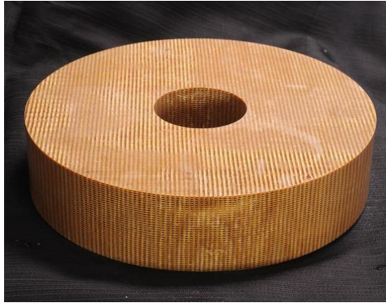
Fig. 2. 9 Quartz fibre 3D woven composite used by NASA for Orion test vehicle [29].
