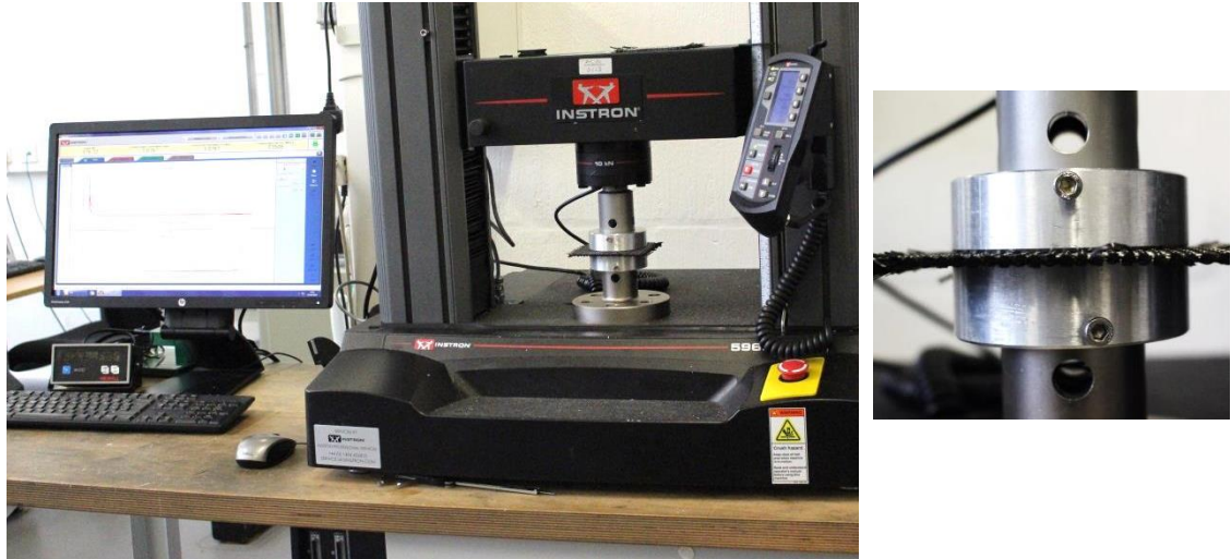
Fig. 4. 1 Instron set-up for compressibility test (left) and the compaction zone (right).
