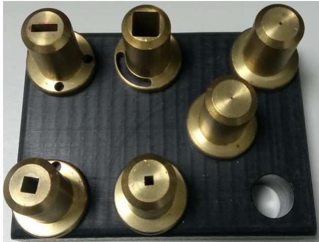
Figure 2.3.1. The standard tertiary collimators for use on the Small Animal Radiation Research Platform (SARRP).
