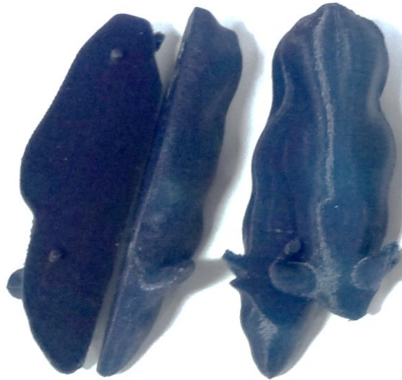
Figure 2.2.3. Sagittal and coronal plane cut models to hold film.
