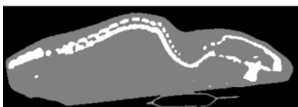
Figure 2.3.5. A CBCT scan of the 3D printed zoomorphic phantom. A CBCT scan of the heterogeneous density model showing the varying density of the skeleton (white) in contrast to the soft tissue (grey). Not shown are the lungs.
