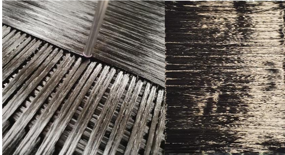
Figure 4-11 Cross-ply [0/90] structure preforming on robotic tow placement developed by the University of Manchester
