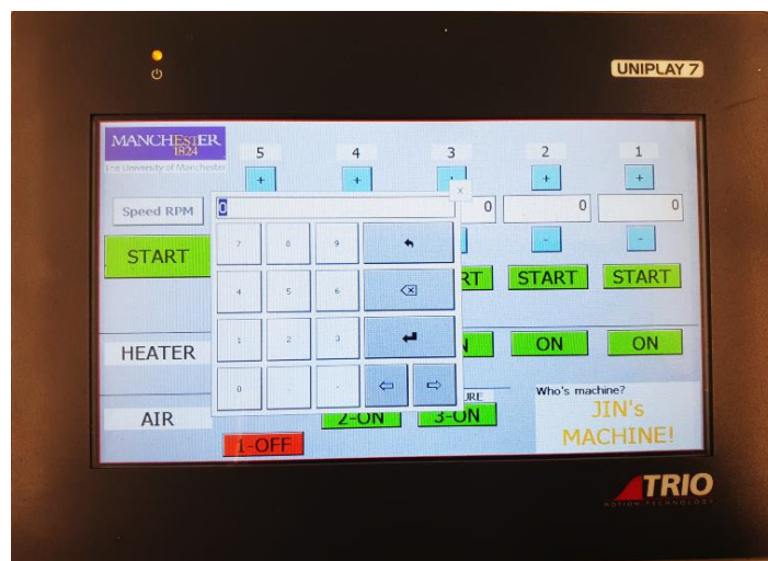
Figure 3-20 (a) display design and function setting for each button in the software and (b) the corresponding display operation mode after uploading the program
