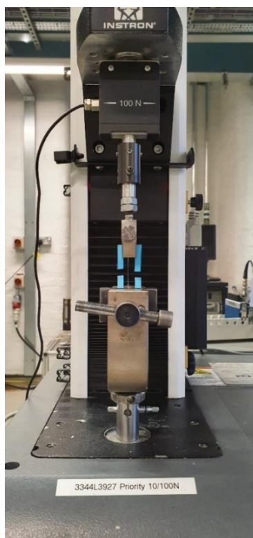
Figure 4-16 Single fibre tensile test set-up on the Instron 3344 with 100N load cell
