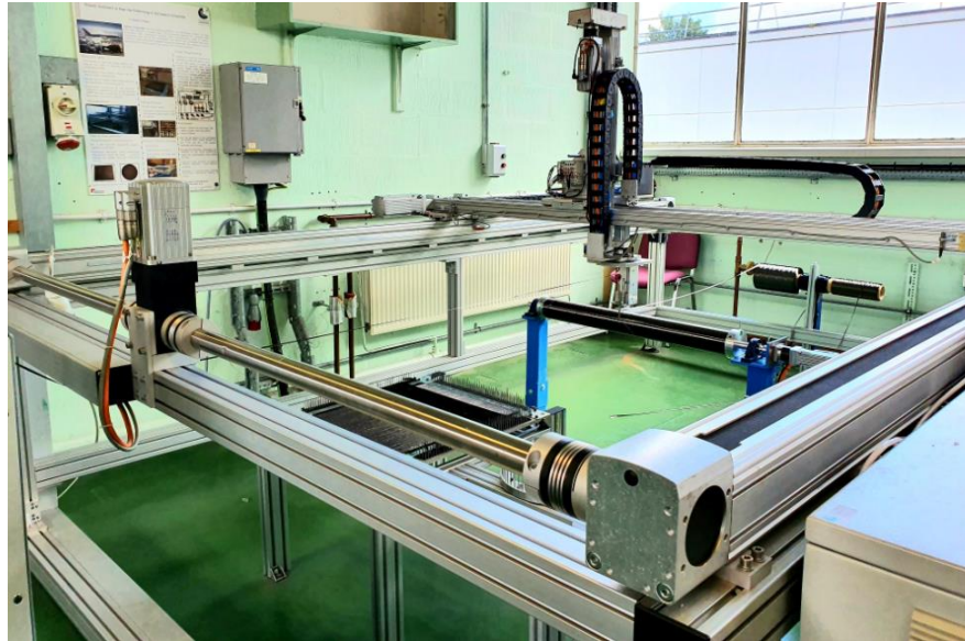
Figure 2-16 Gantry automated fibre placement at the University of Manchester
