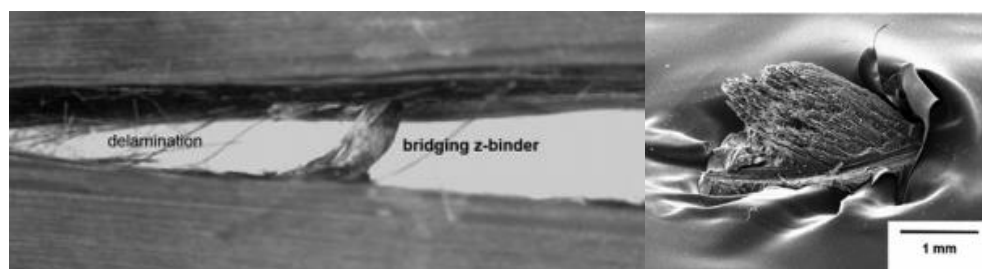
Figure 2-5 (a) Delamination crack and z-binder bridging, and (b) fracture of 3D woven structural composites in mode I test [31]
