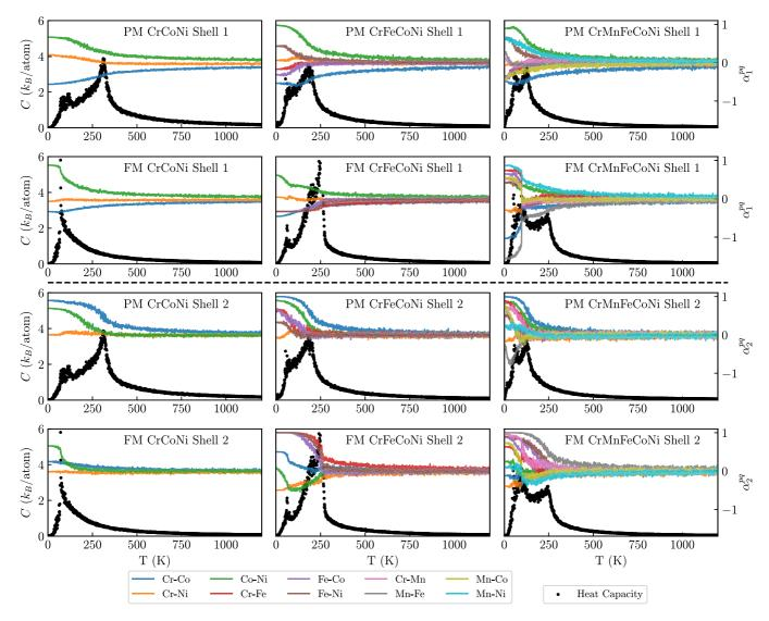
FIG. 4. Plots of the Warren-Cowley short-range order parameters on first and second coordination shells for the three considered systems along with a measure of the system's specific-heat capacity, *C*. Each subplot is labeled to indicate the alloy and magnetic state for which it shows results. The magnetically ordered results show a significant weakening of ordering between Cr and Co and a strengthening of interactions between Fe and the other elements.
