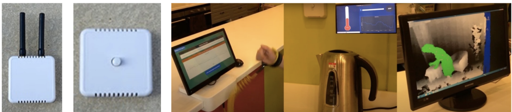
Fig. 2. The a) ‘rabbit ears’ gateway (left), b) ‘little blob poking out’ environmental sensor (middle) and c) Interactive demos of the platform’s capabilities – (i) The wearable, (ii) The environmental sensor and (iii) the Kinect silhouette camera.
