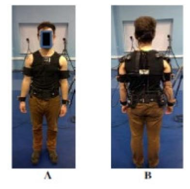
Figure 1. Xsens sensors placement, A) front view, B) back view
