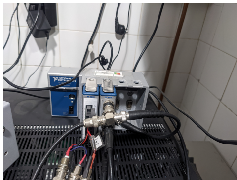
Figure 2.28: Photograph of the National Instruments chassis cDAQ-9177 that contains both an ADC and DAC module.
