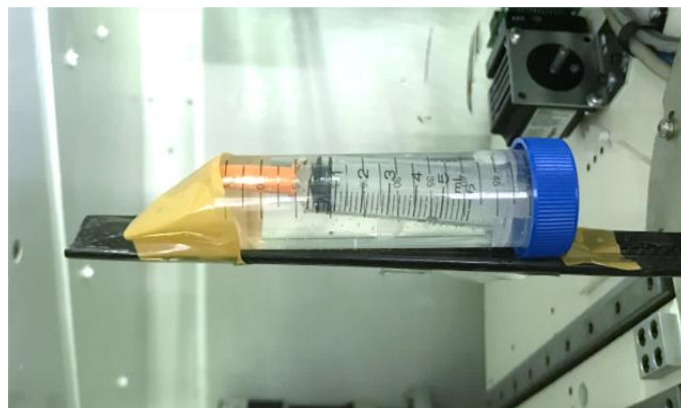
Figure 3.15: Phantom used to simulate a tumour inside a mouse.
