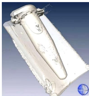
Figure 2.14: Example of a 3D reconstructed acquisition of a water-filled Eppendorf tube used for the FLEX™ Triumph™ equipment's CT camera validation. Inside the phantom, an air bubble detected by the camera can be clearly seen.
