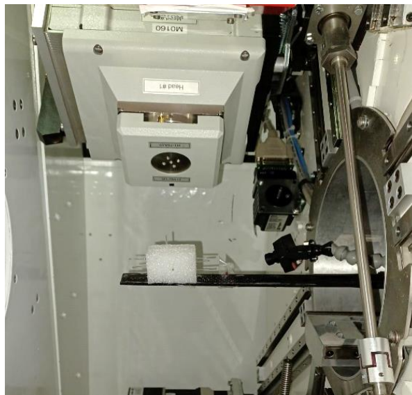
Figure 3.7: Interior view of the FLEX™ Triumph™ equipment. In the Figure, the gamma camera can be seen with the N5F75A10 collimator, prepared to acquire the image of a phantom.
