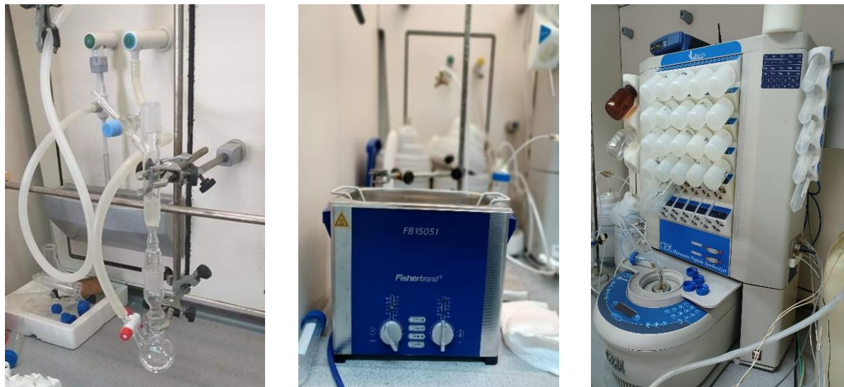
Figure 3.1: Equipment and materials used for all three methods of SPPS. [Left] Assembled reactor for ‘classical’ SPPS. [Centre] Equipment used for US-assisted SPPS. [Right] Equipment used for MW-assisted SPPS.
