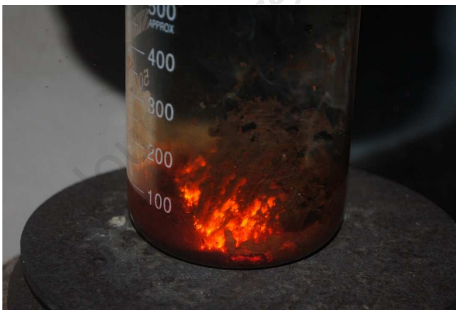
Fig. 1. Photograph of combustion reaction taking place at fuel to oxidant ratio ( \psi ) of 2.0.
