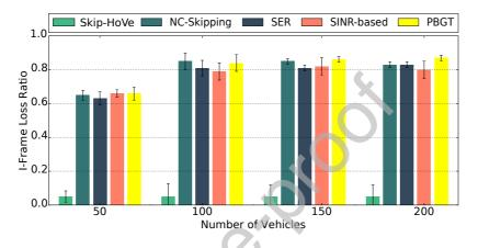
Figure 5: I-Frame loss ratio for videos delivered by different handover algorithms
