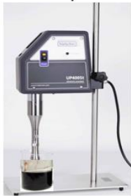
Amplitude 60%, Half Duty Cycle, 2 hrs. Sonication time
