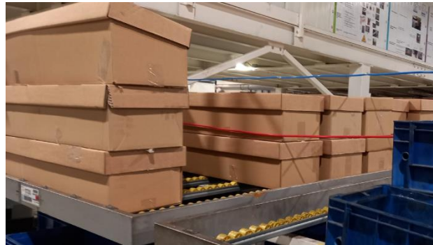
Figure 42 - Height limiter NOK situation
