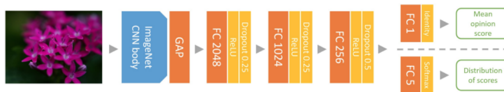
Figure 1. End-to-end architecture of trained KonCept512 model to predict MOS values [9].
