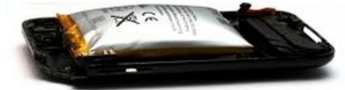
Figure I.9. Swollen Li-ion pouch cell (adapted from [42]).
