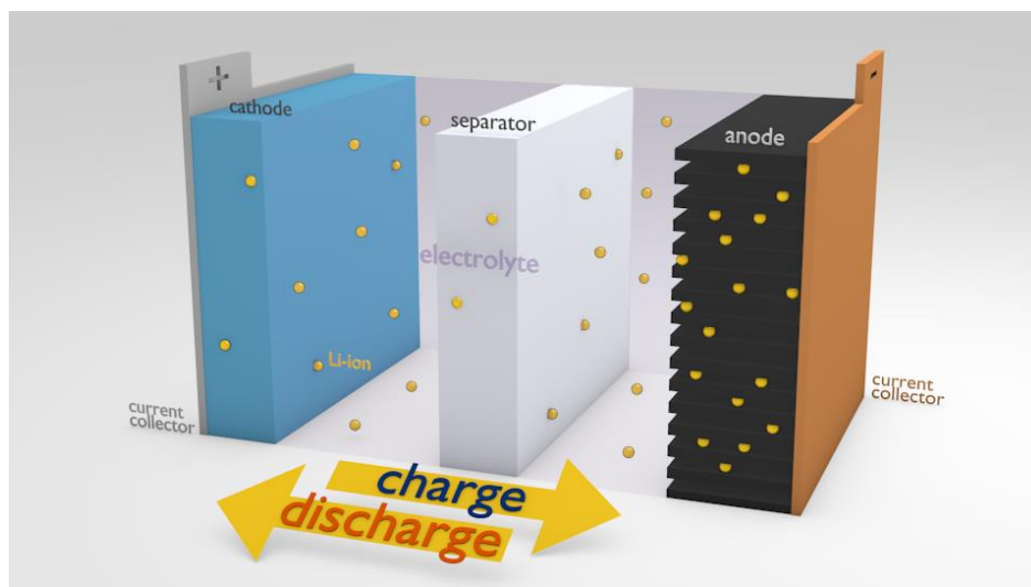
Figure I.5. Ion flow through the LIB separators. These provide a barrier between the anode (negative electrode) and the cathode (positive electrode) while enabling the exchange of lithium ions from one side to the other (adapted from [34]).
