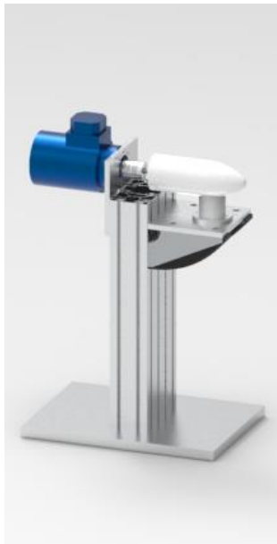
Figure 48 - Rendering of the structure used (including the electric motor and the generator)
