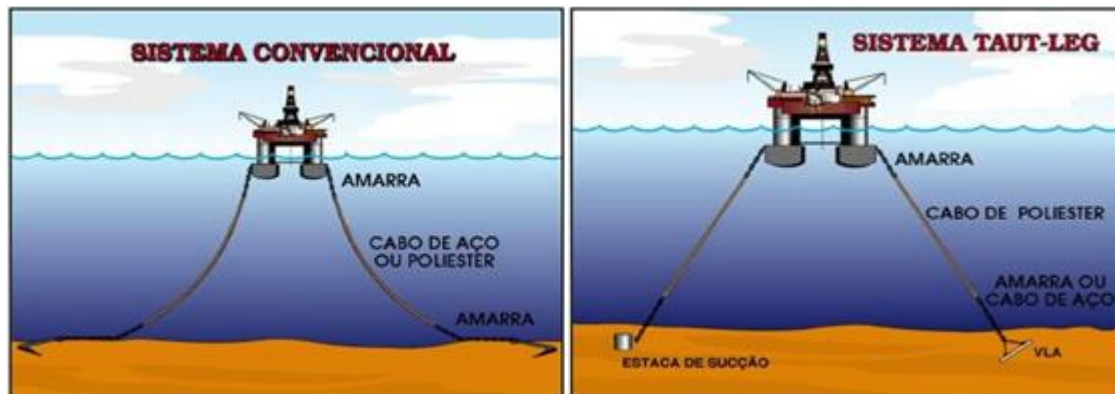
Figure 10 - Mooring in conventional system and TAUT-LEG system [22]
