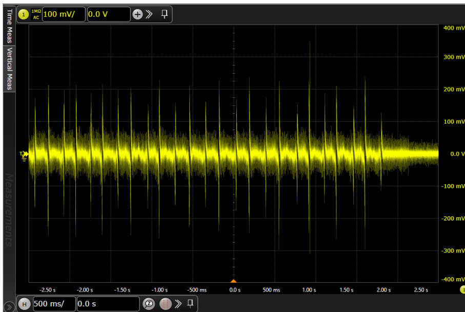
Figure 3.9: Waveform of the voltage produced by the third coil in open circuit taken with oscilloscope DSOS804.
