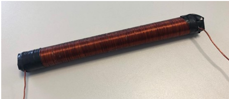
Figure 3.3: Second electromagnetic harvester prototype implemented.
