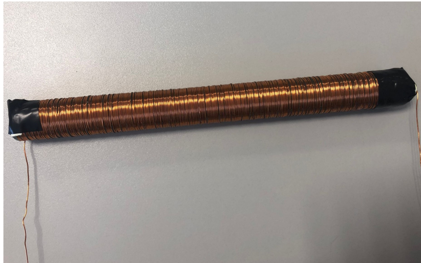
Figure 3.8: Third electromagnetic harvester prototype built.
