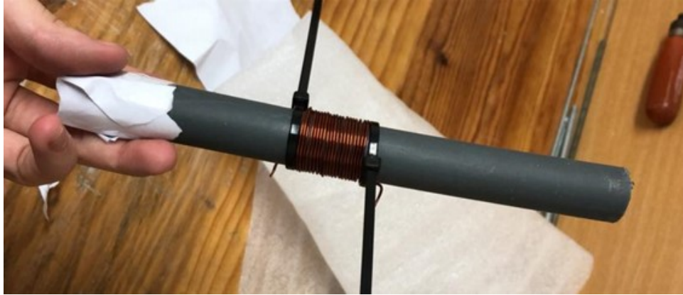
Figure 3.2: First electromagnetic harvester prototype implemented.
