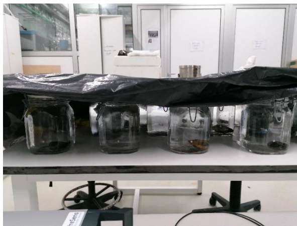
Figure 9. Experimental setup of respirometric chambers for the measurement of respiration rate (RR).
