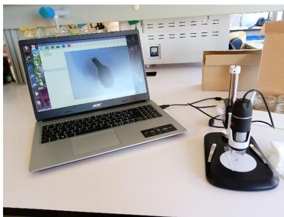
Fig. 18. Method used to monitor planarian Girardia tigrina regeneration. Digital photographs were taken using an USB microscope (1600x).
