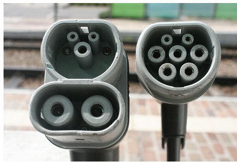
Figure 2.5: Combo 2 (left), compared to IEC Type 2 (right): two large direct current (DC) pins are added below, and the four alternating current (AC) pins for neutral and three-phase are removed [14]
