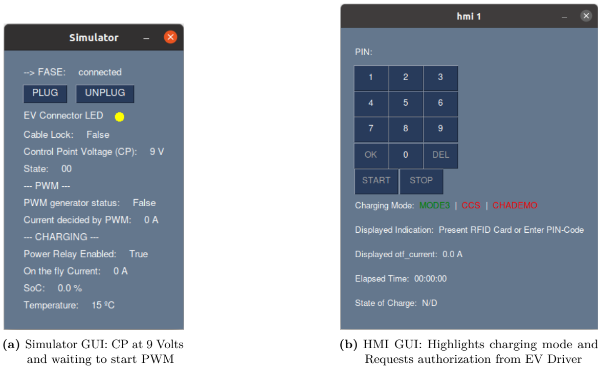
Figure 4.5: Simulator and HMI: EVPlug
