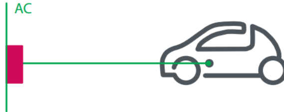
Figure 2.6: Mode 1: Household socket and extension cord [6]
