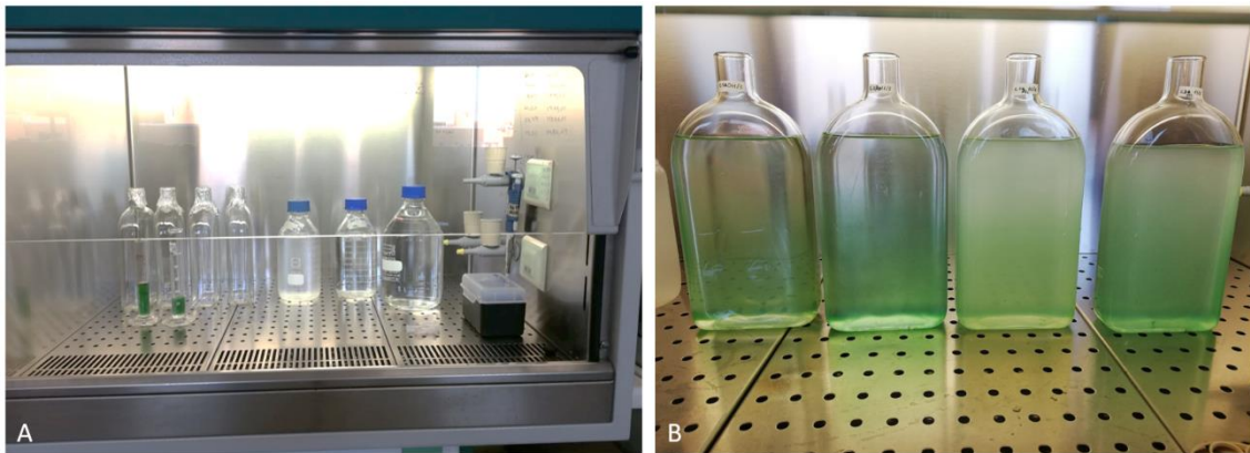
Figure 6 Inoculation of A. platensis cultures: A - culture flasks, medium, pipet, pipet tips and measuring cylinders inside the Laminar Flow Chamber; B - culture flasks after inoculation, for maintenance (from left to right: two flasks of strain 1 in SM and 2 flasks with JM).
