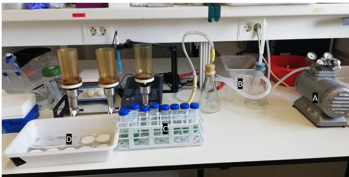
Figure 7 Filtration set: A- vacuum pump; B- filtration flasks; C- dilutions of culture; D- glass microfiber filters.
