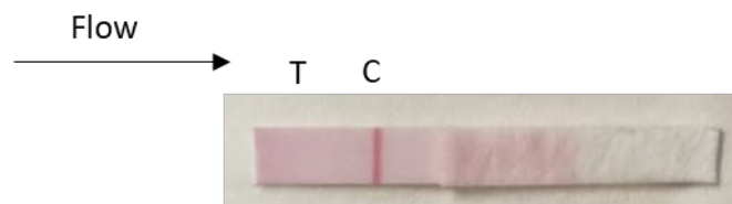
Figure 6.4: The blank test: the testing was done with no PCR product, this was done to validate the test and the results expected were a negative test.
