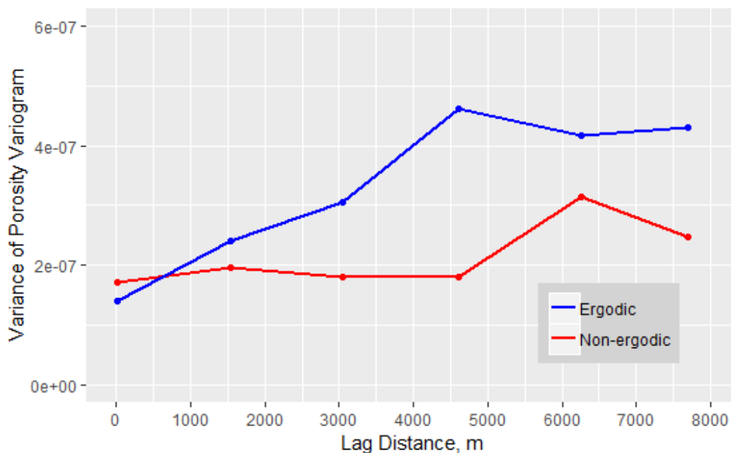
Figure 17: Uncertainty (Variance) in the directional (90°) variogram of Agbabu porosity data – DBSCAN-aided technique
